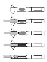
Bend the borders of the channels round with flat pliers. Then bend the plates around the insulation and finally put the sockets into the connector so that the locks would lock on and cannot be pulled out again. If there is resistance, gently try to lift the lock on the connector with a tip. Not too much, otherwise it will stay open forever. Lean the tip at the edge of the socket and gently move it forward. You probably used too much tin or bent the borders too little.
