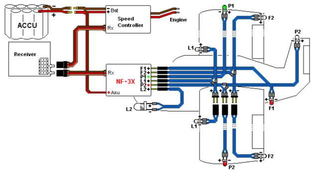
A short-term short circuit at a unit output does not harm the circuit thanks to the current outlets. The circuit regulates the current by burning the voltage difference between the supply voltage and the necessary voltage for diodes in the transistor. The worst condition for the unit is the case when the circuit is supplied by high voltage and short circuit at the output occurs. In that moment, the entire power (the passing current x power supply voltage) changes to heat in the transistor.
