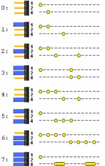
Both circuits anti-collision lights flash every one second. With the blue couplers (jumpers) **1**, **2**, **4** you can select one of eight combinations of flashes. Sum for of connecting jumpers determines the number of combination.
