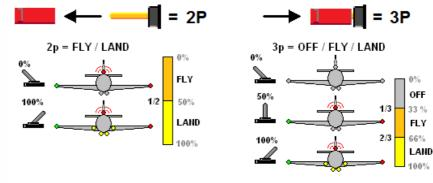
In 2P mode position and anti-collision lights are on continuously and landing lights are controlled from the transmitter. The 3P mode is the standard range of servo divided into thirds. In the first lights are switched off, in the second position lights and anti-collision lights are switched on, in the third all the lights are switched on.
