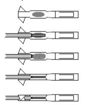
Bend the borders of the channels round with flat pliers. Then bend the plates around the insulation and finally put the sockets in the connector so that the locks would lock on. If there is resistance, gently try to lift the lock on the connector with a tip. Not too much, otherwise it will stay open
